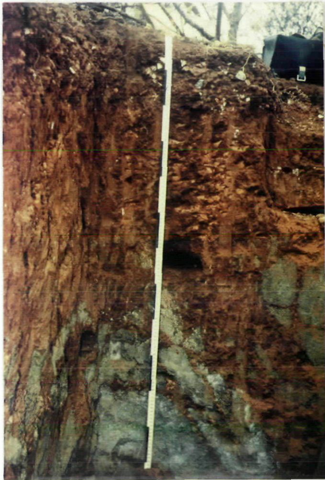
Photograph N°1. Truncation and surface in profile EAK/51. Only the B horizon remains, resting directly on Pre-cambrian rocks.
