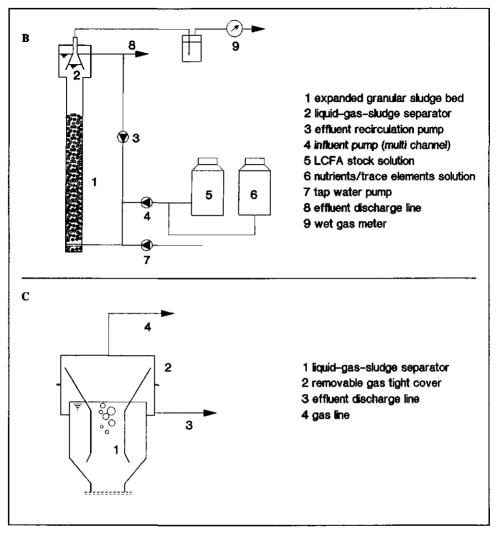
Figure 1b. Schematic representation of the set-up used for digestion of capric and lauric acid (experiments 2-4). The EGSB reactor used in experiment 2 is shown. Figure 1c. The modified gas-liquid-solids separator used in experiments 3 and 4.
