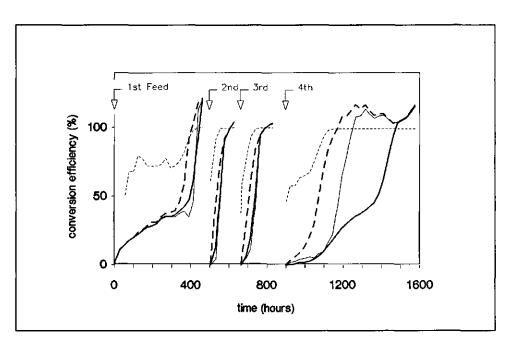
Figure 1. Simulation of UASB reactor start-up (experiment A; -- capric acid removal; -- capric acid degradation  $(f_g)$ ; -- acetate formation  $(f_2)$ ; -- methanogenesis; c.f. equations 1-6 and Table 1)
