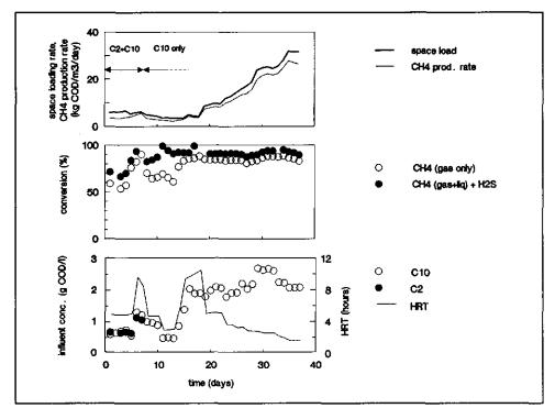
Figure 3. Results obtained with anaerobic digestion of capric acid in an EGSB reactor (experiment 2)
