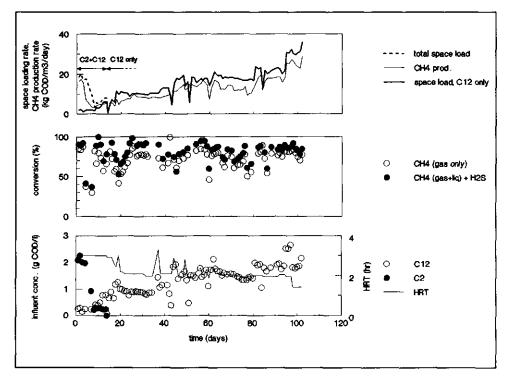
Figure 5. Results obtained with anaerobic digestion of lauric acid in an EGSB reactor (experiment 4)
