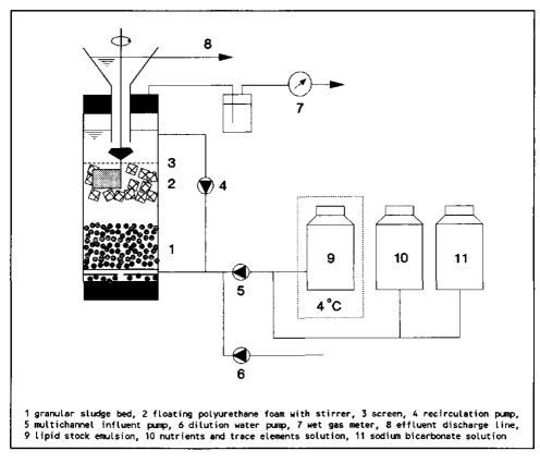
Figure 1. Schematic representation of the hybrid EGSB reactor
