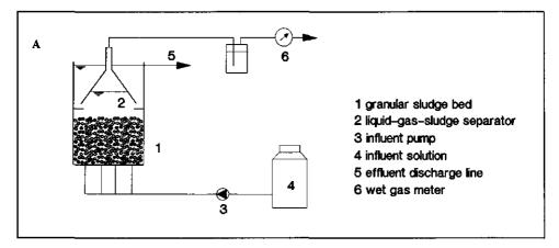
Figure 1a. Schematic representation of the UASB reactor with four inlet points used in experiment 1 (digestion of capric acid)
