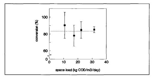
Figure 6. Conversion efficiency of lauric acid in an EGSB reactor as a function of the space loading rate (experiment 4; average;  $\mapsto$  standard deviation; ... average over entire period)
