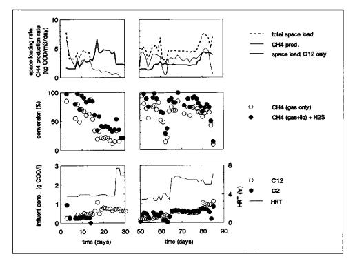
Figure 4. Results obtained with anaerobic digestion of mixtures of capric and acetic acid in a UASB reactor (experiment 3; days 1-15:  $C_{12}$ : $C_2$  0.65; days 50-86  $C_{12}$ : $C_2$  1.12; ratios on COD basis)
