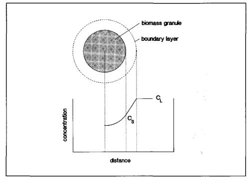
Figure 3. Schematic representation of the model describing transport of capric acid from the solution to the biomass granules, and inside the granules
