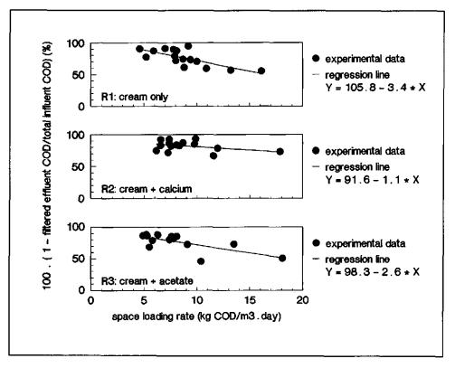
Figure 3. COD removal efficiency as a function of the space loading rate in EGSB reactors equipped with sieve-drum separators. (Note: for reactor 3 the efficiency and space loading rate are based on the cream only, c.f. Table 1).
