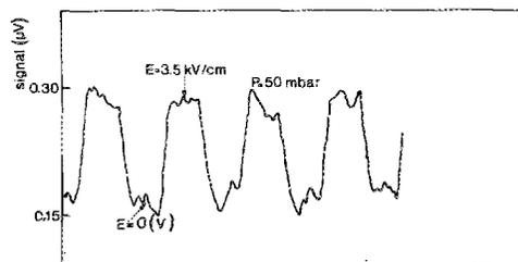
FIG. 2. Stark signal of  $\text{NH}_3$  obtained at 10R(6)  $\text{CO}_2$  laser line at the total pressure of 50 mbar and the electric field strength of 3.5 kV/cm.
