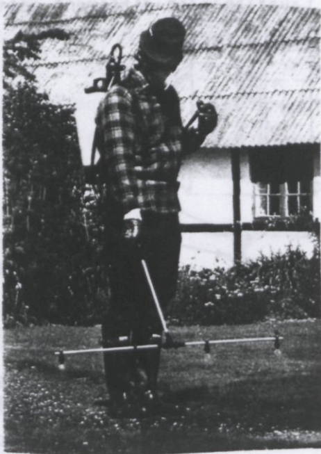
Figure 22. A boom with several nozzles 34 cm apart, instead of a lance for surface treatment.
