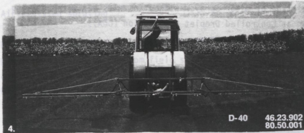
Figure 34. Simple tractor-mounted sprayer with a tank from 200 liters upwards and a boom length from 6m upwards.
