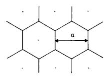
Fig. 2.4b. Tree in a triangular espacement and their theoretically crown  $0.5a^2\sqrt{3}$ . In a profile diagram in principle crown diameter a will be drawn.
