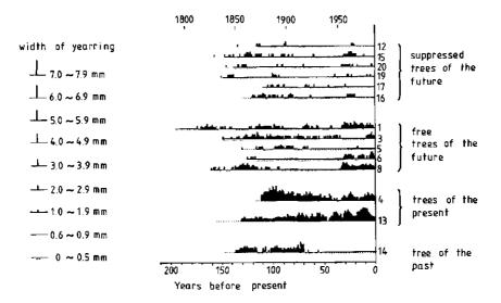
Fig. 3.4. Growth of trees higher than 5 m. Horizontal lines indicate increment cores taken at 50 cm height, while the width of the year-rings is shown vertically above the lines.
