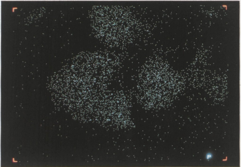
Fig. 8. X-ray element map of phosphorus from the same area as shown in Fig. 2.
