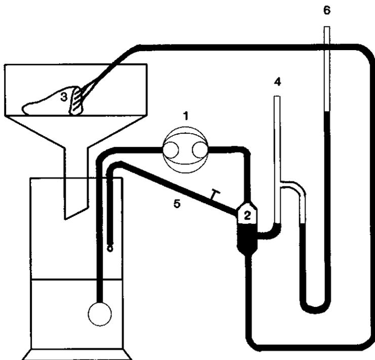
Fig. 2.1 Schematic presentation of the perfusion during the recirculation step with collagenase. The buffer is pumped by a peristaltic pump (1) via the oxygenator (2) to the liver sample (3), which is placed in a Büchner funnel. Oxygen is added via the oxygenator at (4) and escapes via the overload (5). The pressure is monitored with the manometer (6). All vessels containing buffer solutions, the oxygenator and the tubing are placed in a waterbath (40 °C).
