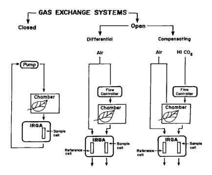
Figure 2.2. Three basic types of gas-exchange measurement systems (redrawn from Field et al., 1989).
