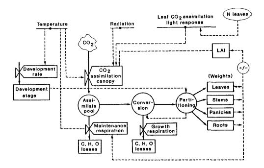
Figure 6.1. A schematic representation of the model ORYZA1. Boxes are state variables, valves are rate variables, circles are intermediate variables. Solid lines are flows of material, dotted lines are flows of information.
