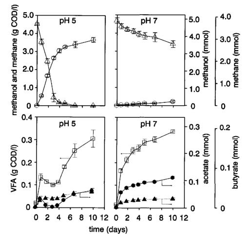
Figure 2 - Methanol degradation, methane and VFA production from freshly sampled reactor microflora in batch experiments. Symbols: △, methanol; ○, methane; □, VFA; △, butyrate; ●, acetate.
