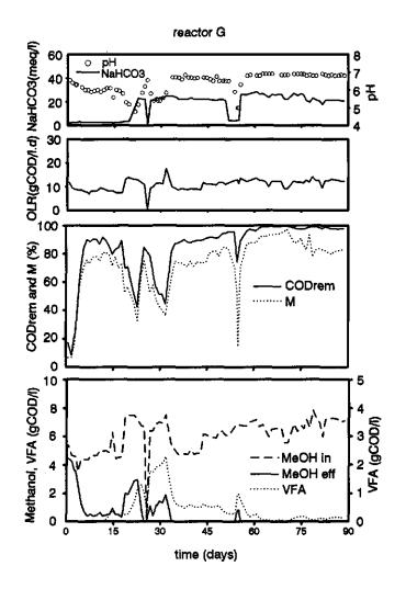
Figure 4 - Operational and efficiency parameters during the anaerobic treatment of methanol in the reactor G (NaHCO<sub>3</sub>, variable). OLR, CODrem and M: same definitions as in Figure 1.
