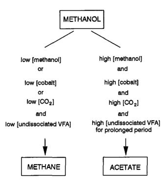
Figure 1 - The final fate of methanol in anaerobic bioreactors.
