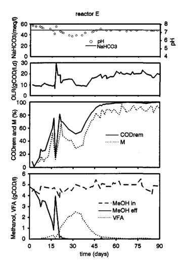
Figure 2 - Operational and efficiency parameters during the anaerobic treatment of methanol in the reactor E (50 meq NaHCO<sub>3</sub> · 1<sup>-1</sup>). OLR, CODrem and M: same definitions as in Figure 1.
