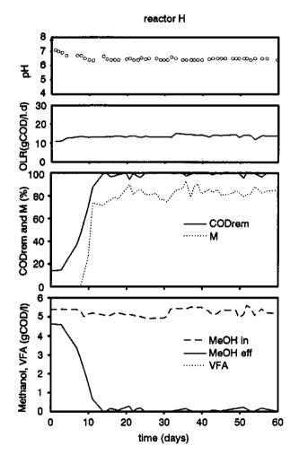
Figure 5 - Operational and efficiency parameters during the anaerobic treatment of methanol in the reactor H (K<sub>2</sub>HPO<sub>4</sub>), 20 meq · 1<sup>-1</sup>; NaHCO<sub>3</sub>, no addition). OLR, CODrem and M: same as in Figure 1.
