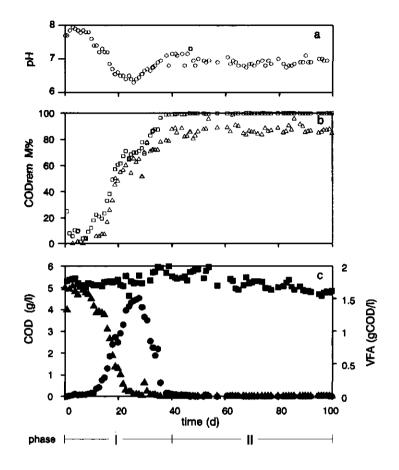
Figure 7 - Operational and efficiency parameters during the anaerobic treatment of methanol in the UASB reactor B. (a) pH; (b) COD<sub>rem</sub> (% COD<sub>in</sub> removed) and M% (Methanogenesis = % COD<sub>in</sub> converted into methane); and (c) VFA, Methanol-COD<sub>in</sub>, and Methanol-COD<sub>eff</sub>. Symbols: see Fig. 6.
