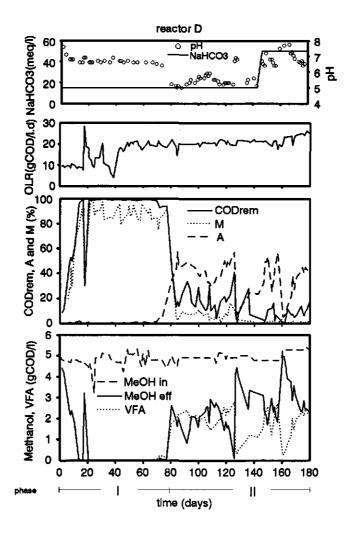
Figure 1 - Operational and efficiency parameters during the anaerobic treatment of methanol in the reactor D (initially 15 meq NaHCO<sub>3</sub> · 1<sup>-1</sup> and later 50 meq NaHCO<sub>3</sub> · 1<sup>-1</sup>). OLR = COD influent applied per liter reactor per day; CODrem = methanol removal - acetogenesis; A (Acetogenesis) = % COD influent present as VFA in the effluent; M (Methanogenesis) = % conversion COD influent to methane.
