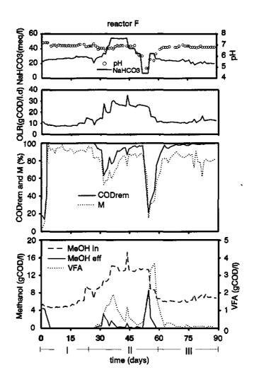
Figure 3 - Operational and efficiency parameters during the anaerobic treatment of methanol in the reactor F (NaHCO<sub>3</sub>, variable). OLR, CODrem and M: same definitions as in Figure 1.
