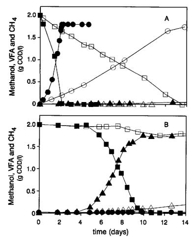
Figure 2 - Cummulative methane and VFA production from methanol. (A) No inhibitor was applied; (B) with BESA. Symbols: ○ methane (no cobalt); ● methane with cobalt added; □ methanol (no cobalt); ■ methanol with cobalt added; △ VFA (no cobalt); ▲ VFA with no cobalt added.
