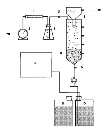
Figure 2 - Schematic diagram of the UASB reactor used in this study. a: COD influent; b: nutrients; c: nitrogen; d: sampling point; e: sludge bed; f: effluent; g: gas sampling point; h: NaOH; i: lime soda pellets; j: gas meter.
