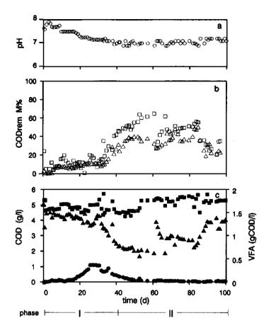
Figure 6 - Operational and efficiency parameters during the anaerobic treatment of methanol in the UASB reactor A (Co deprived column). (a) pH; (b) COD<sub>rem</sub> (% COD<sub>in</sub> removed) and M% (Methanogenesis = % COD<sub>in</sub> converted into methane); and (c) VFA, Methanol-COD<sub>in</sub>, and Methanol-COD<sub>eff</sub>. Symbols: ○, pH; □, COD<sub>rem</sub>; △, M%; ●, VFA; ■, methanol-COD<sub>in</sub>; △, methanol-COD<sub>eff</sub>.
