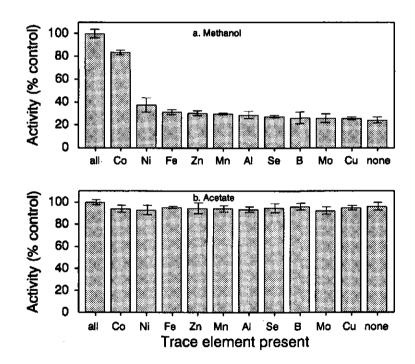
Figure 3 - Influence of individual trace element on methanogenesis. (a) methanol, (b) acetate. Only one trace element is present. Activity is expressed as a percentage of a control where all trace elements were present.
