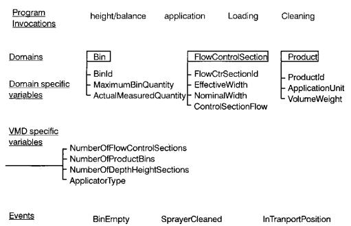
Figure 7. An agricultural sprayer descibed as a Virtual Manifacturing Device
