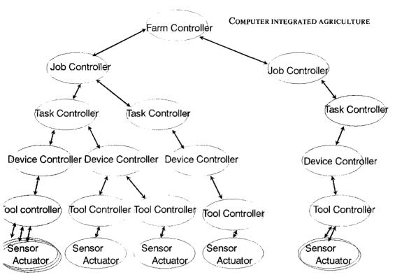
Figure 6. A controll architecture in primary farm production
