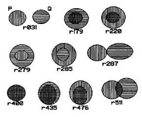
Figure 4.7 Topologic relationships between two area objects
