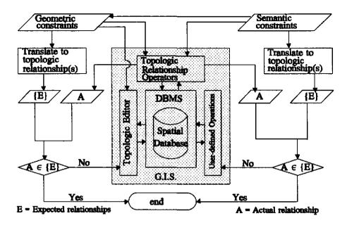
Figure 5.3 Scheme for consistency operations in vector maps
