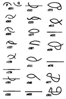
Figure 4.9 Topologic relationships between two line objects
