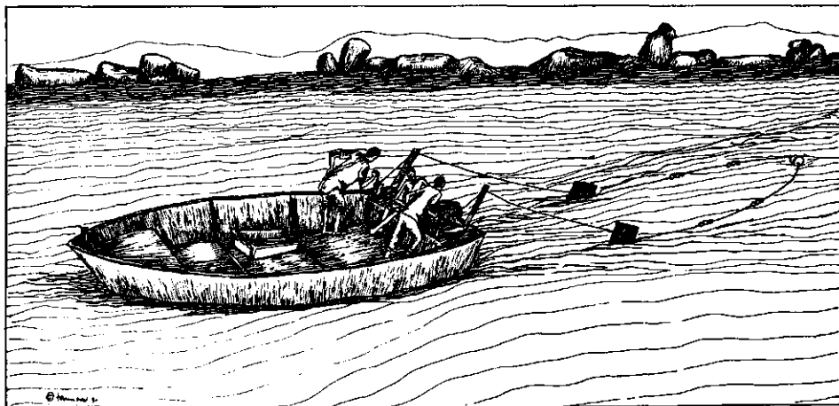
Figure 4.22 Shooting/hauling the bottom trawl of a small, outboard engine powered trawler.
