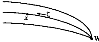
Figure 2 The coordinate \xi is taken along the streamline through the point x .
