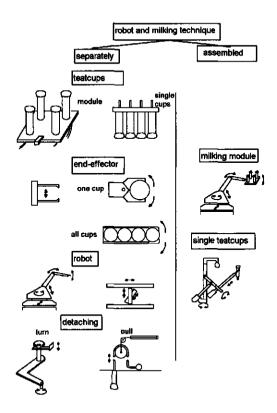
Fig. 2. An automatic milking system assembly
