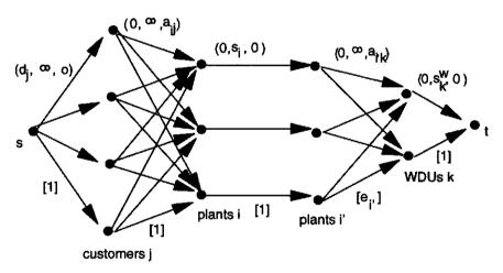
Figure 3.2: The minimum cost network flow problem with losses.
