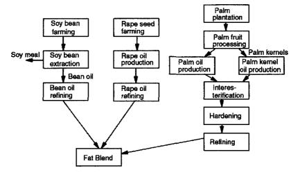
Figure 5.2: Example of a process tree for a fat blend for margarines
