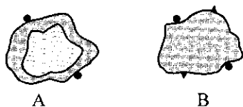
Figure 11.2. (A) A solution species has reacted with the surface of the original solid (hatched part) to form a coating (dotted part) of a new phase (shrinking core), the species is also adsorbed on the coating. (B) A solution species has completely converted the original solid to form a solid solution. Adsorption of species (● and ▲) that are constituents of the solid solutions takes also place.
