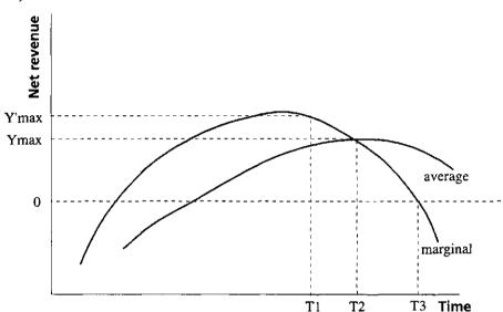
Figure 7.1 Determination of the optimal time for replacement in a situation without an alternative opportunity (T3), and in situations of identical replacement (T2) and nonidentical replacement (T1) (derived from Van Arendonk, 1985)
