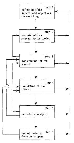
Figure 5.1 The basic steps of systems simulation
