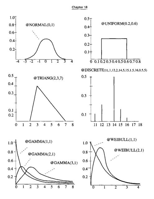
Figure 18.2 Example probability distribution graphs (normal, uniform, triangular, discrete, gamma and Weibull)
