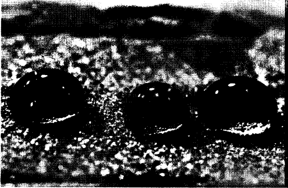
Fig. 1.2 Water repellency measurement (WDPT test) by placing three drops of water upon the surface of a soil sample and determining the time to complete absorption.
