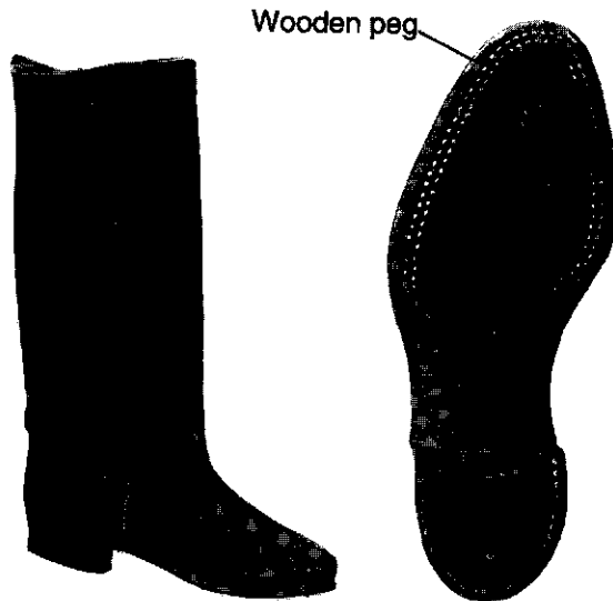
Figure 4.3: A leather boot from ca. 1910 (collection Museum of footgear, leather and leatherware in Waalwijk). The sole is nailed to the upper part with wooden pegs that swell in contact with water, making the boot almost waterproof. According to W. Blok (personal communication) one pair of these boots must have cost a two-and-a-half month wage of a workman. In current prices, this is at least 2,000 Dutch guilders (ca. 1,000 U.S. dollars).
