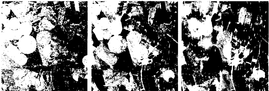
Figure 3.7: JPL-AIRSAR data (June'91, Barrax area around the ITAP center) with from left to right C-, L- and P-band respectively. Clearly the effects of the pivot irrigation can be seen as also the tracks of the tires within the irrigation fields.
