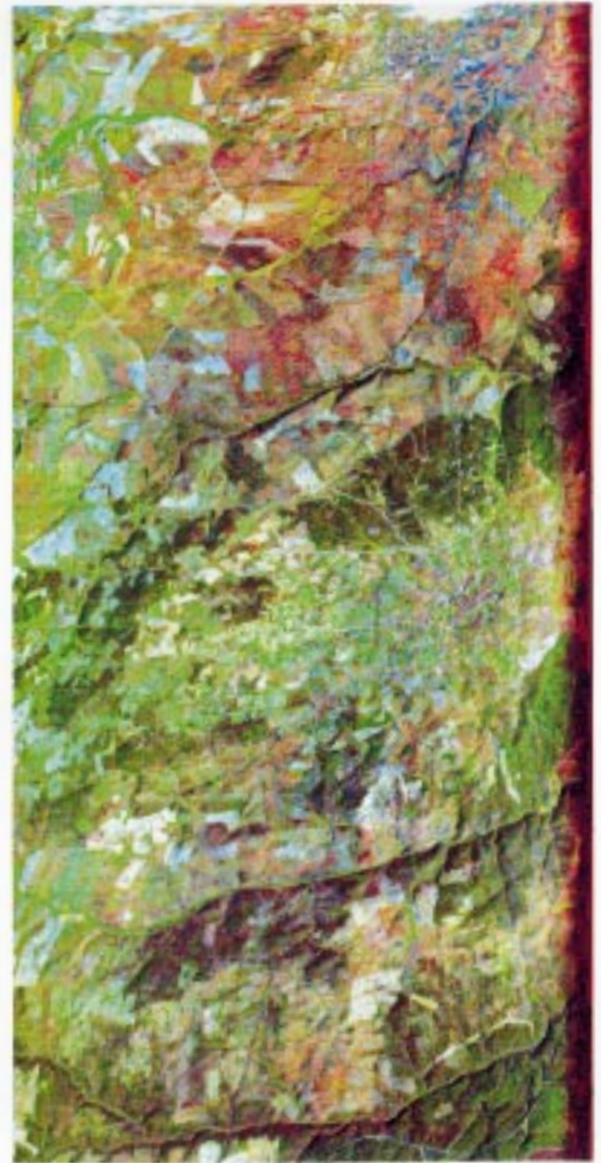
Figure 3 Color composite image of GERIS bands 35, 26, and 4 displayed in RGB with decorrelation stretching applied.
