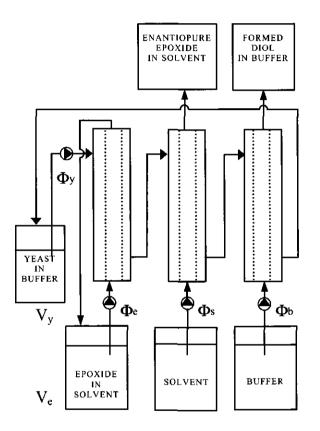
Scheme 3. Schematic diagram of a two-phase cascade membrane bioreactor for continuous extractive epoxide resolution.
