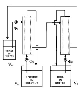
Scheme 2. Schematic diagram of a two-phase cascade membrane bioreactor for batch-wise epoxide resolution.
