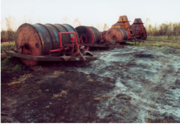
Figures 2.5 Equipment used by the cutting method: pneumatic-combine and peat compactor
