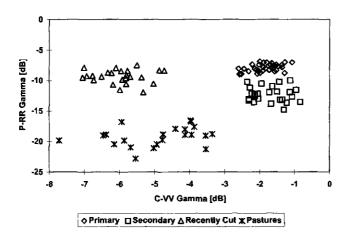
Figure 2.4. Scatter plot of the C-VV and P-RR field averaged backscatter levels for all 105 fields in the 45°-50° incidence angle range, for the four main land cover types
