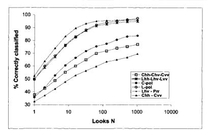
Figure 2.5. Overall Maximum Likelihood (ML) classification accuracy (expressed in percentages) at the 95% level of confidence for the  $45^{\circ}-50^{\circ}$  incidence angle range for several combinations as function of the speckle level expressed in number of looks.
