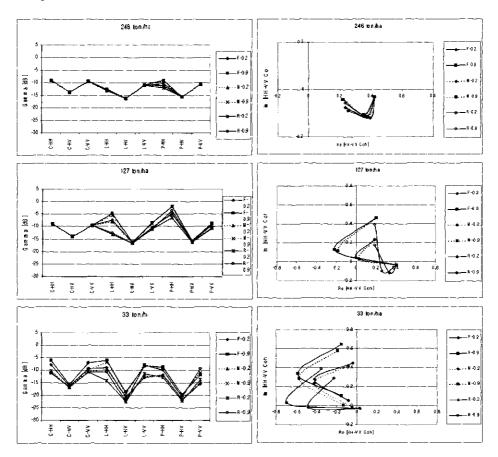
Figure 5.9. Intensity signatures and polarimetric coherence signatures for selected plots of the HD-15 data set, for high, intermediate and low biomass levels. Each plot presents signatures for 3 terrain roughness conditions (F, M, R) and two different extreme soil moisture conditions (0.2 and 0.9).
