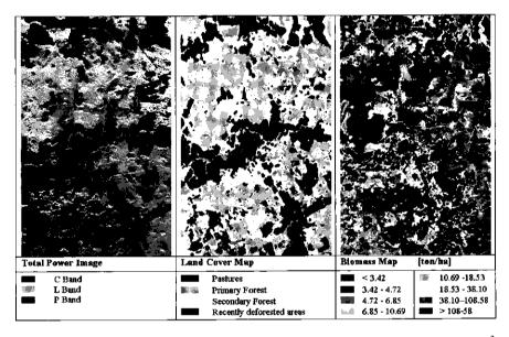
Figure 2.8 (a) AirSAR Total Power image, (b) Land Cover map and (c) Biomass map for a  $4 \times 7 \text{ km}^2$  area in Guaviare. In the biomass map the areas of recently cut forest are masked (black) .(see colour plate 1).
