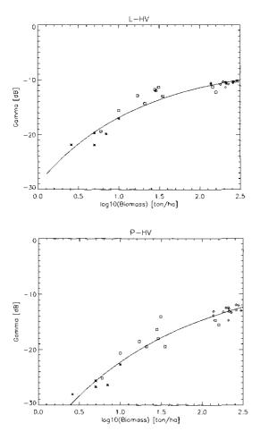
Figure. 2.6. L-and P-band backscatter with HV-polarisation as function of biomass. The biomass is the fresh weight above ground biomass (in ton/ha) on the logarithmic scale (i.e. 1.0 is 10 ton/ha, 1.5 is 31.6 ton/ha, etc.). Experimental data for primary forest ( $\Diamond$ ), secondary forest ( $\Box$ ) and pasture (\*) are fitted to a curve of the form  $\gamma_i$  [dB]=  $a \exp(bx) + c$ , where x is the logarithm of the biomass.
