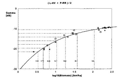
Figure 4.3. (PRR+L HV/2)-polarisation average as function of biomass for the Guaviare site. The biomass is the fresh weight above ground biomass (in tons/ha) at the logarithmic scale (i.e. 1.0 is 10 ton/ha, 1.5 is 31.6 ton/ha, etc.). Experimental data for primary forest ( $\diamond$ ), secondary forest ( $\Box$ ) and pasture (\*) are fitted to a curve of the form  $y[dB] = a + b(1-\exp(-cx))$ , where x is the logarithm of the biomass.
