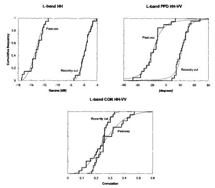
Figure 2.3 Theoretical cumulative probability density distributions of L-band HH-polarised backscatter, HH-VV phase difference and correlation, respectively, compared with experimental observation (step-functions). For recently cut areas the K-S fit significances Q are 0.9995, 0.81 and 0.85, respectively, and for pastures 0.96, 0.82 and 0.9996, respectively
