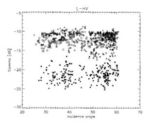
Figure 2.2 L-band HV-polarised field averaged backscatter levels as a function of incidence angle for the four main land cover types: primary forest ( $\diamond$ ), secondary forest ( $\Box$ ), recently cut forest ( $\Delta$ ) and pasture (\*).
