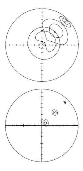
Figure 3.3. Confidence intervals for the complex coherence at 50% and 90% for (left) 14-look and (right) 280-look samples, for a phase difference of 45°, and  $|\rho_i|$  values of 0.1, 0.5 and 0.9. The intervals are drawn within the unit circle of the complex plane
