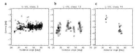
Figure 3.2. L-band VV-polarized plot averaged backscatter as a function of incidence angle, for three examples.a) class 3, b) class 13 and c) class 14.
