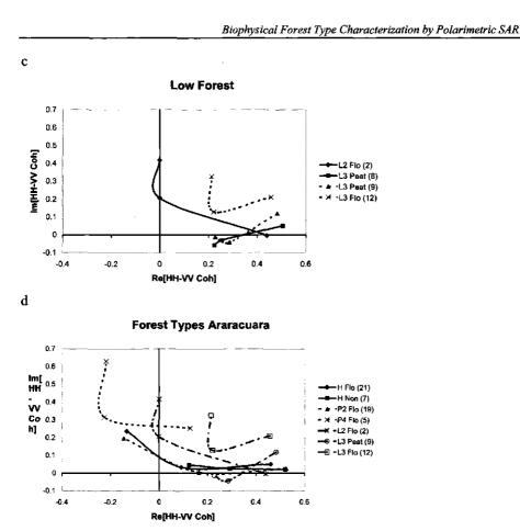
Figure 3.6. Multi-frequency complex coherence curves for (a) high forest, (b) flooded palm forest, (c) low forest and (d) different forest types (see also Figure 7). The curves connect the C-band coherence (in these examples always the right-most point), with the L-band and the P-band value (at the other end of the curve). In the legends plot numbers are shown within brackets, furthermore, H= High forest, P= Palm forest, L= Low forest, Flo= flooded, Non= non-flooded.
