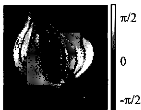
Figure 2.6. Phase image of a tulip bulb. The image is the first echo out of a CPMG echo train of 46 echoes.
