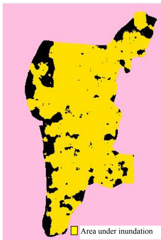
Figure 9.14 Drainage inundation without structure control (1:10 year return period with 3 days consecutive rain)
