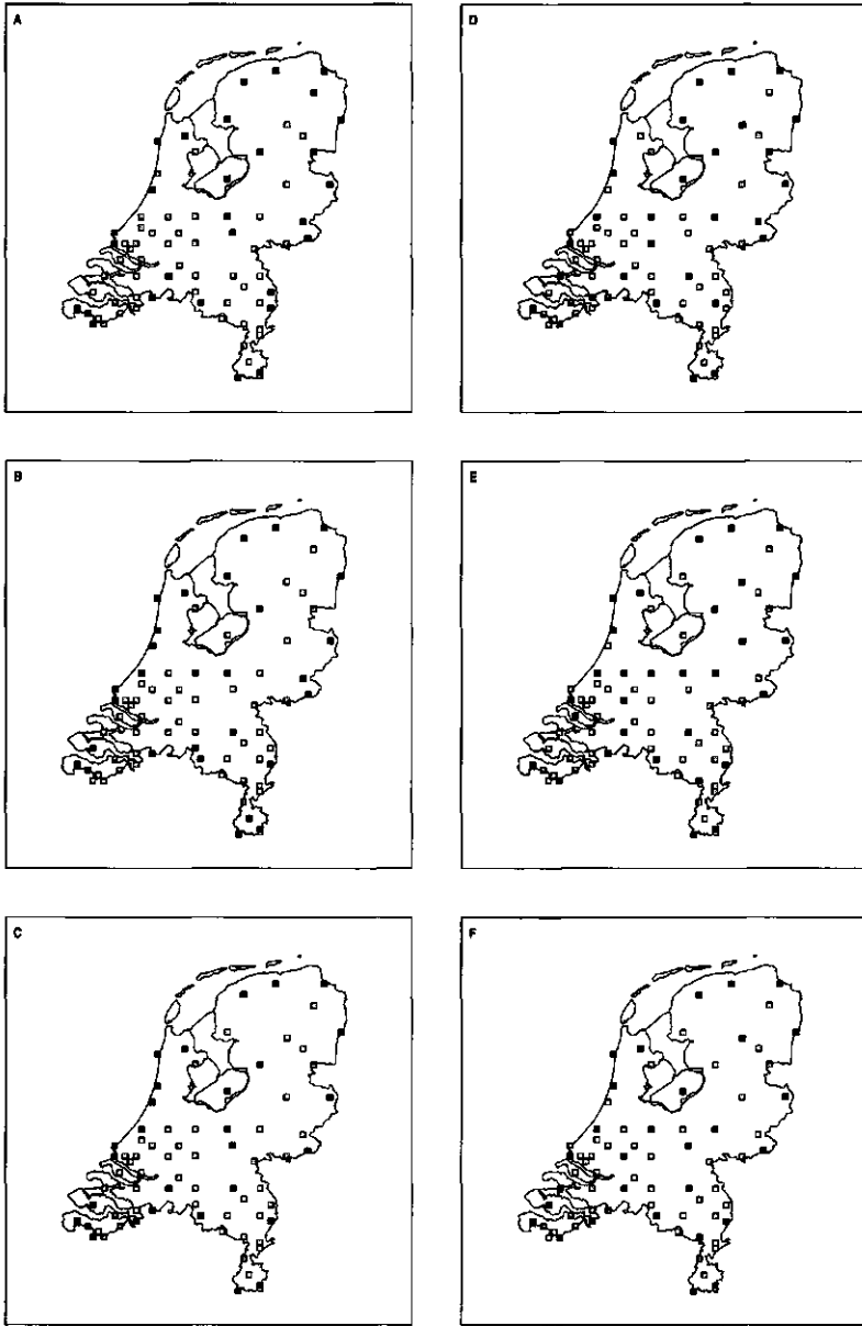
Figure 5.6: Monitoring networks (black squares) obtained from the network of 74 monitoring stations by the drop-add algorithm ( n = 29, m = 6 ). Tricube weight function, p = 1 , anisotropic and h_f = 120 (km), for the three design criteria in Section 5.2.4, (A-C). Same for McLain weight function, h_f = 136 (km) (D-F).
