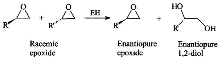
**FIG. 1.1. ENANTIOSELECTIVE ENZYMATIC HYDROLYSIS OF A RACEMIC EPOXIDE TO ITS VICINAL DIOL AND ONE REMAINING EPOXIDE ENANTIOMER**
