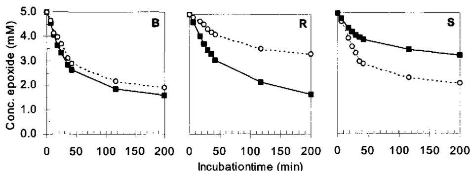
FIG. 5.2. TIME COURSE STUDIES OF THE HYDROLYSIS OF ( $\pm$ )-1,2-EPOXYOCTANE USING NON-IMPRINTED AND IMPRINTED EH-POLYMERS
