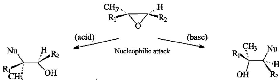
FIG. 1.2. NUCLEOPHILIC RING-OPENING OF EPOXIDES ARE STEREOCONTROLLED
