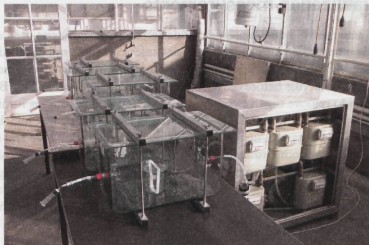
Picture 1. Glass compartments and pump used for volatilization experiments. On the left side the air-inlet with active coal filter. A petri-dish is placed on a glass beaker for measurement of tri-allate volatilization from a glass surface.
