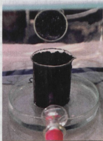
Picture 4. Glass Beaker with soil in the compartment. On the background the air-inlet with stainless steel sponge. On the foreground the air-outlet.
