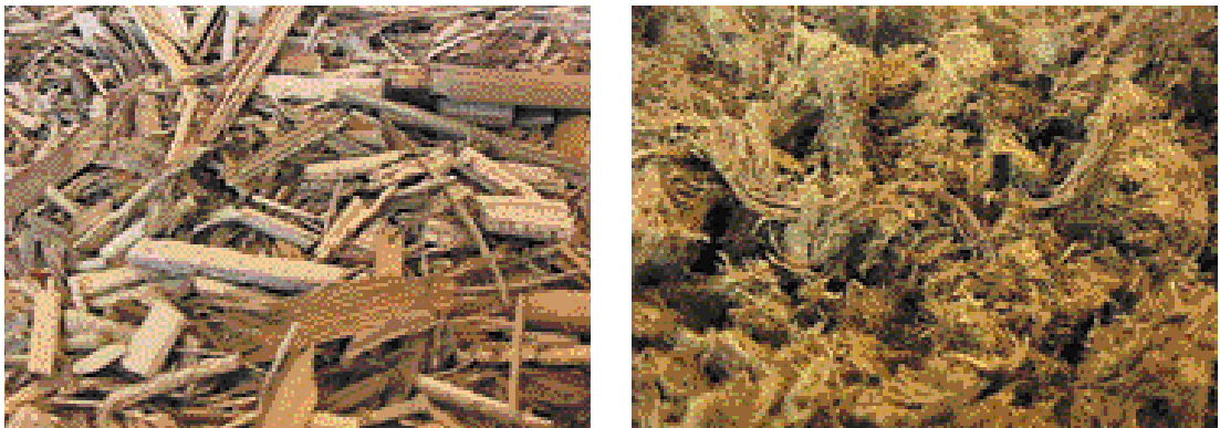
Figure 4. Chopped Miscanthus before (Left) and after extrusion in combination with a sodium hydroxide treatment (Right). The pretreatment removed 77% of the lignin.
