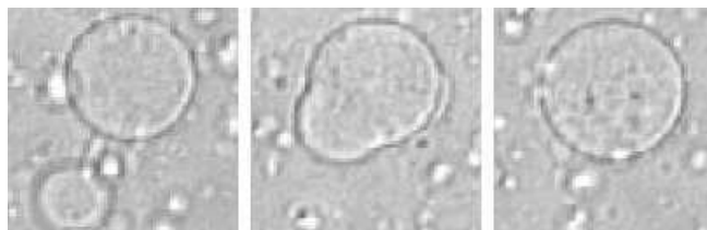
Figure 7.6: Fusing DOPG giants upon osmotic inflation after dehydration in a hypertonic glucose solution ( \Delta c = 200 mM). The photographs were taken two minutes apart.
