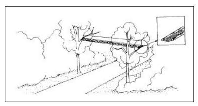
Figure 14. A rope-bridge crossing a road to facilitate a save passage for red squirrels (Source: Bekker 2002)
