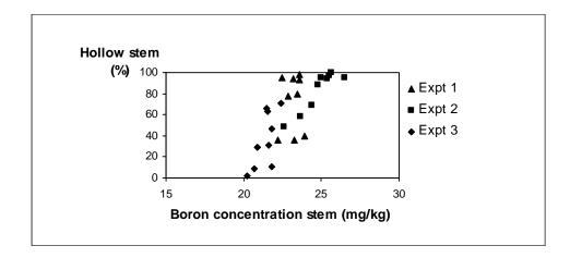
Fig. 1. The relation between the percentage plants with a hollow stem and the Boron concentration of the stem.
