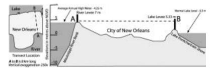
Figure 2: Profile of New Orleans from Lake Pontchartrain to Mississippi River (adapted from New Orleans US Army Corps of Engineers).
