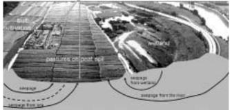
Figure 10: Soil subsidence causing land level decline due to drainage of pastures on peat soil, resulting in high pumping costs, the decline of wetland quality and damage to buildings
