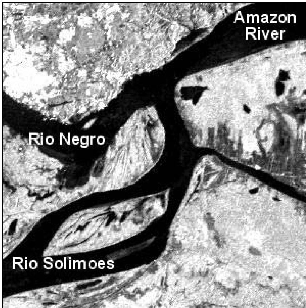
Figure 3.19: Non-forest class: Rio Negro (north) and Rio Solimoes (south) becoming Amazon rivers and characterized by low backscattering values ( DN=30 , \sigma^0 = -18.99 ). Image area: 30 \times 30 \text{ km}^2 .
