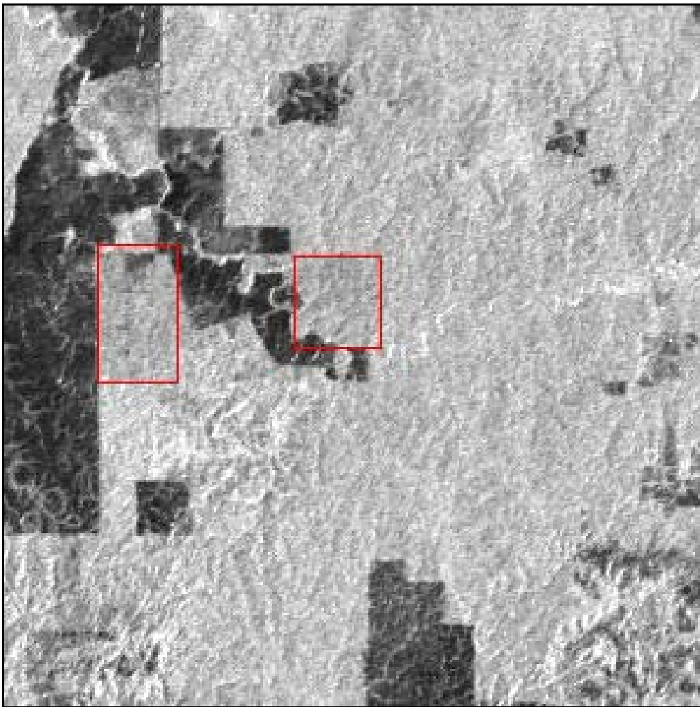
Figure 3.16: Degraded forest class: abandoned pasture with partial re-growth forest in the 2 red boxes ( DN=100 , \sigma^0 = -8.54 ). Image area: 30 \times 30 \text{ km}^2 (see color Figure B.9 - Appendix B, pp. 207).
