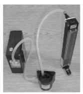
Figure 3 Attach flowmeter and sampling pump to RespiCon stage flow checker
