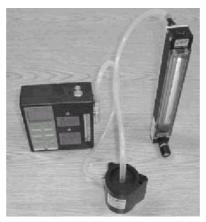
Figure 2 Attach flowmeter and sampling pump to RespiCon total flow checker
