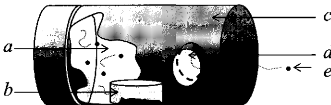
Figure 1. Cylinder used to test repellent effect of dry conidia of the entomopathogenic fungus Metarhizium anisopliae to female mosquito Anopheles gambiae s.s. (bioassay1). (a) plastic cylinder containing adult mosquitoes; (b) Petri-dish containing dry conidia; (c) dark cloth covering the cylinder; (d) exit hole from which mosquitoes can escape (e). NB Exit hole is connected to a 30 x 30 x 30cm netting cage (not shown).
