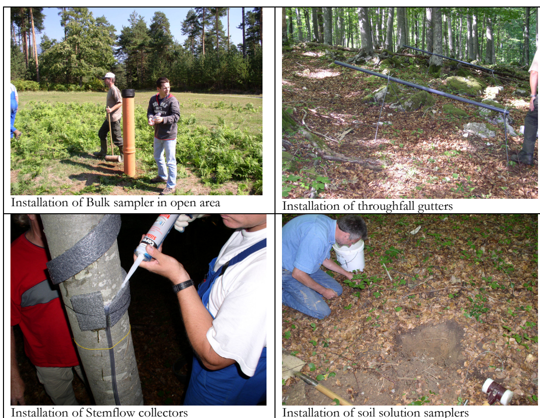
Figure 7. Photos of installation of bulk sampler, throughfall gutters, stemflow collector and soil solution samplers
