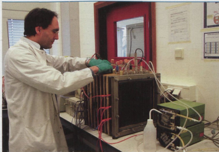
Direct production of electricity out of wastewater using microbial fuel cells (TNO).
