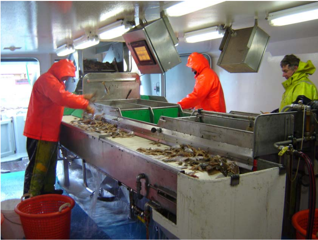
Figure 8: Fish processing line onboard PT1
