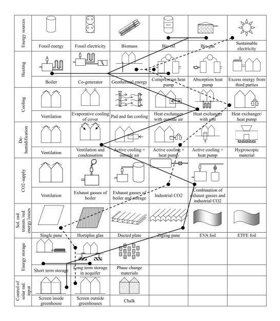
Fig. 1. A morphological diagram; concept 1 (dashed line) and concept 2 (solid line) of a minimum fossil energy greenhouse.
