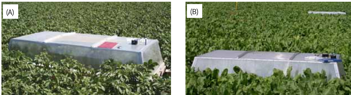
Figure 7 Flux chamber placed on permanently installed frames. (A): Potato field (Langeweg); (B): Field with sugar beets (Vredepeel)
