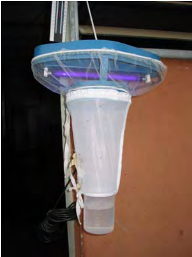
Figure 9. OVI UV light trap:Gold standard method for sampling crepuscular and nocturnal biting Culicoides at livestock
