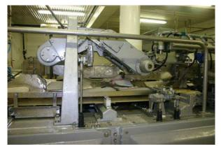
Figure 3 Machine filleting cod
