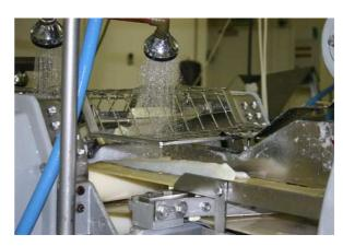
Figure 4 Machine filleting cod
