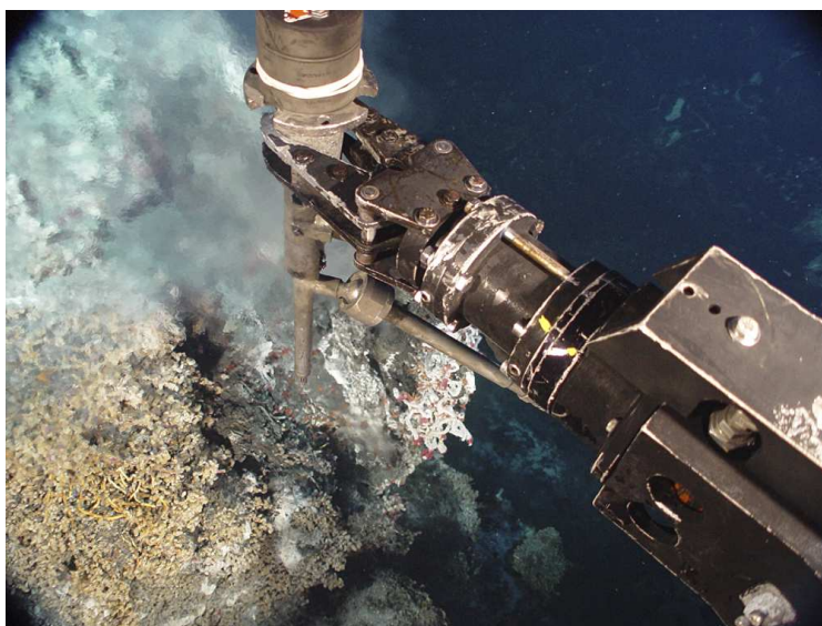
Figure 10.1 Remotely Operated Platform samples vent fluids from the Northeast Pacific Ocean (Photo: NOAA, http://oceanexplorer.noaa.gov )
