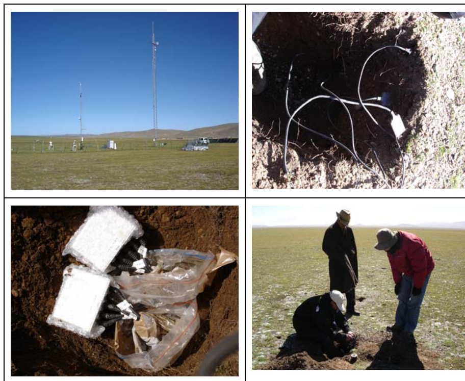
Figure 5. Soil moisture sensors installed at the BJ-Site in Naqu on the Tibetan plateau
