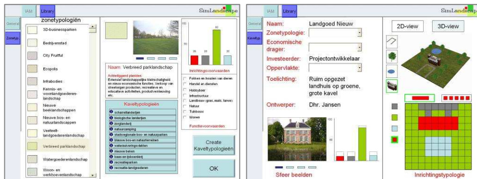
Figure 7: in the library with cadastral typologies, existing parcel typologies can be assembled or new typologies can be created in a user-friendly editor
