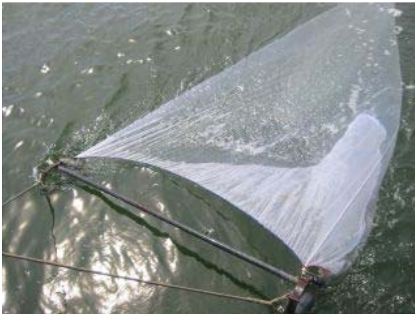
Figure 3 2 m beam trawl net used to fish on epifauna and juvenile fish (mesh size 1 cm 2 ).
