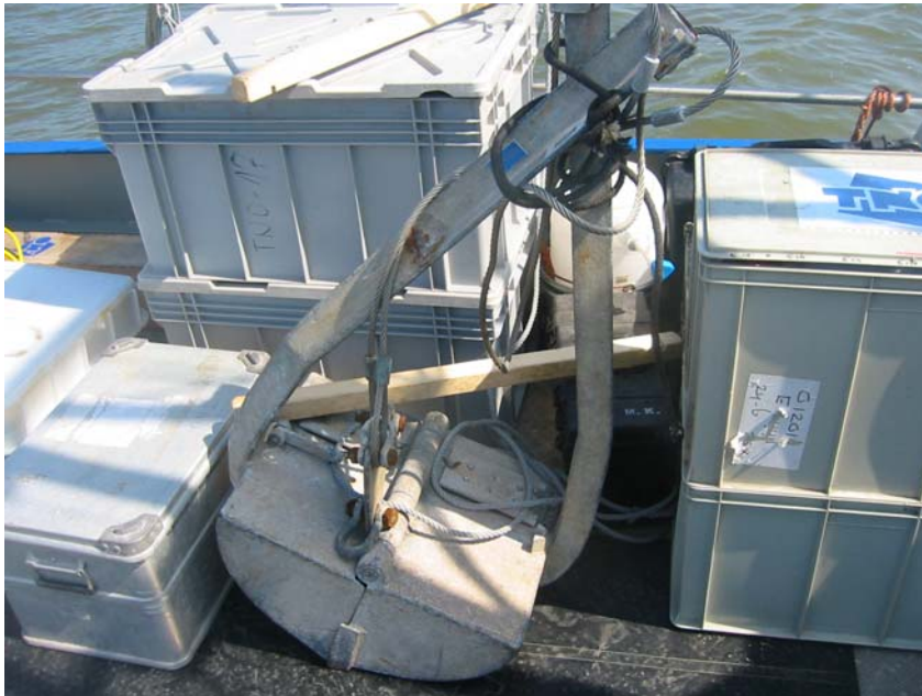
Figure 2 Van Veen grab used to ground truth the seabed (0.1 m 2 ).
