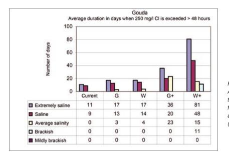
Figure 12: Average duration in days that 250 mg/l Cl is exceeded for longer than 48 hours at Gouda (Source: Beijk, 2008)
