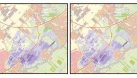
Figure 16: Illustration of inundation simulation after a breach in the dike by the river Hollandsche IJssel by Moordrecht
