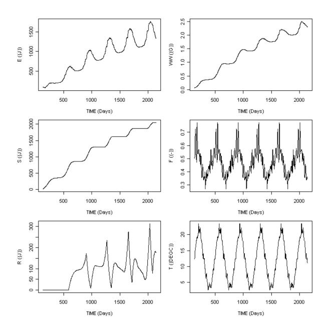
Figure 33 Evaluation of the output of the DEB model for the Eastern part of the Oosterschelde. Variables plotted are (E) Energy in reserves, (S) Energy in structural body mass, (R) Energy in reproductive organs, (WW) Total wet weight, (F) scaled functional response and (T) water temperature.
